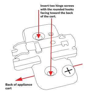
**STEP 15:** To attach the soft-close hinge, snap one hinge at a time onto the hinge mounts, hooking the front hook first, then pushing down the back until you hear a click. This may take multiple tries, and you may need to loosen the adjustment screw.
