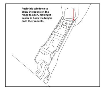
Pushing this tab while trying to snap the hinge on will help the hinge have enough clearance to snap into place.
