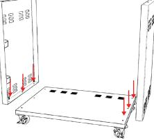
**STEP 4:** Attach Bottom Back Panel - The bottom back panel is first secured to the bottom cart panel with screws. (The bottom of the panel has openings for screws to go through; see the diagram.) The number of screws used varies by the size of the grill cart you are assembling. Attach but do not tighten. Next, secure the back panel. Attach to side walls before adding top bar.
