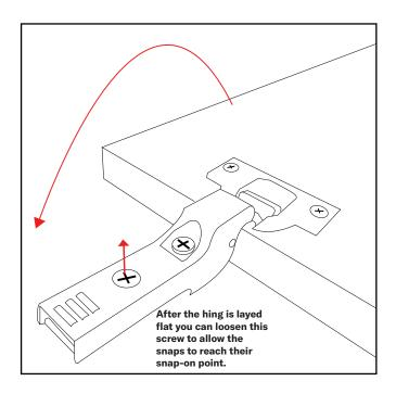
**STEP 14:** To attach the soft-close hinge mounts to the cart as shown.
