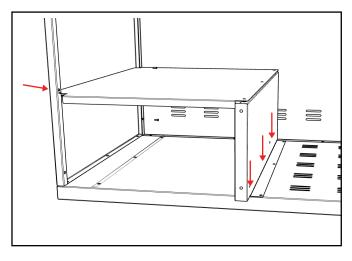
**STEP 9:** Attach the right-side drawer slide to the lower right side of the cart.
