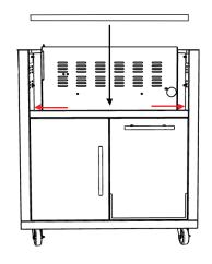
**STEP 17:** Attach side shelves - four screws per shelf are used to attach them to the right and left side panels. Both shelves are exactly the same and can be used on either side. Start all four screws into the side panel, as the shelf can then simply be placed over the screws and pushed downward into place. Once in position, tighten completely.
