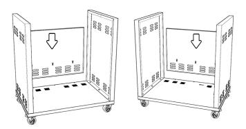
**STEP 5:** Attach the upper two screws on the back side panel, but do not fully tighten them until the cart is fully assembled. Then attach the side panels to the lower back panel.
