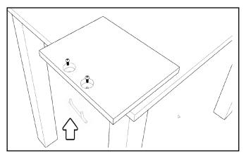
**STEP 12:** To attach the soft-close hinges to the cart, start by flattening the hinges and loosening the adjustment screw.
