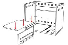
**STEP 8:** Attach the shelf to the interior of the appliance cart using six screws: three on the interior of the cart and three on the exterior.
