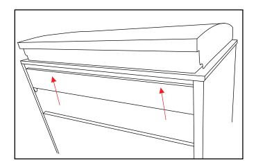
**STEP 20:** Put locking screws in each side of the back panel.
